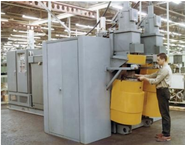
Fig 4 - One of the first EBW units supplied to the auto industry.
