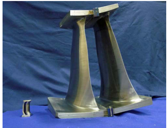
Fig. 2 W501F Vane Segments After EB Welding
