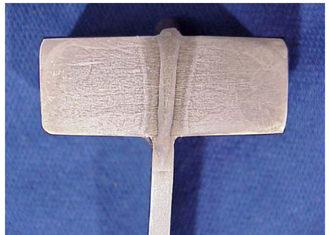
Fig. 6 EBraze™ Joint in a Compressor Cover
